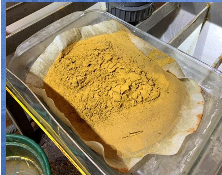
Gold Sludge from Electrowinning Cell Assayed @ 98.648% Gold
